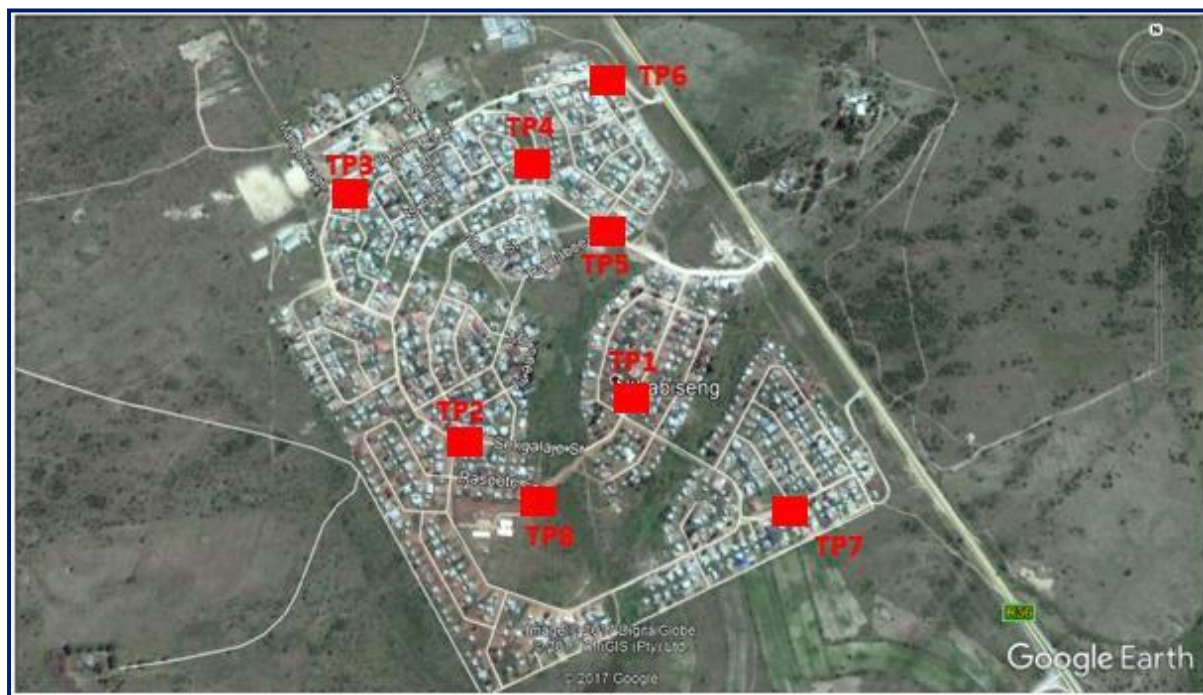
Figure 2: Centerline survey Test pit location along the streets
